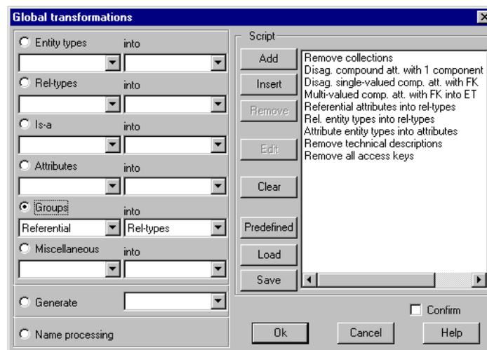
**Figure 8-3:** The *Basic Global transformation* assistant of DB-MAIN showing a simple transformation script for COBOL conceptualization. The *Advanced Global transformation* assistant includes user-defined predicates, filters and loop control structures as well as user-defined predicates and operations libraries.
