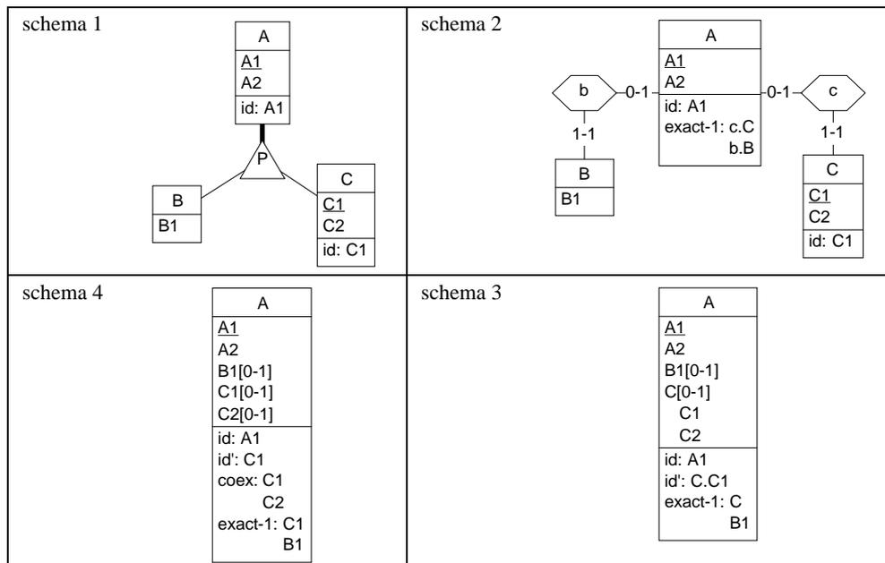
**Figure 2-7:** A complex schema transformation. First, the ISA relation is transformed through **ISA-RT**. Then, subtypes are transformed into attributes (**ET-Att**), which in turn are disaggregated (**Dis-agg**).
