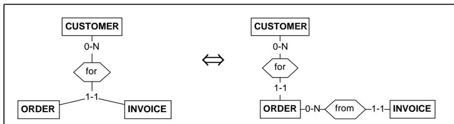
**Figure 6-4:** A record hierarchy implemented as a record sequence. In the left-side schema, a sequence of interleaved ORDER and INVOICE records depend on each CUSTOMER record. This interleaving structure implements an ORDER-INVOICE hierarchy.
