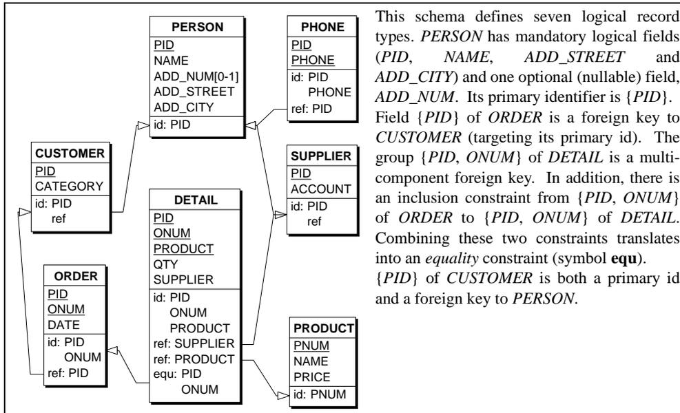
**Figure 2-2:** Abstract logical structures. This relational schema is an approximate translation of the schema of Figure 2-1. The term record type must read *table*, field must read *column* and primary id must read *primary key*.
