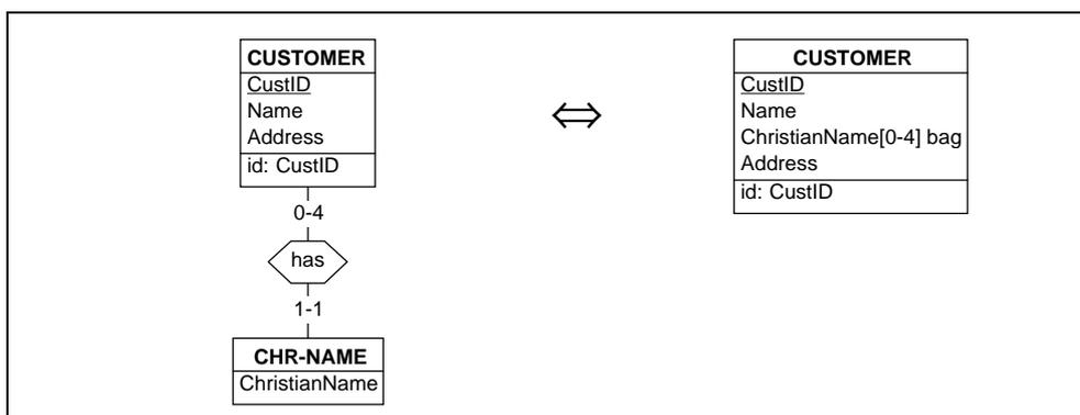
**Figure 7-5:** Recovering a multivalued attribute. Since entity type CHR-NAME has no identifier, it has been transformed into a bag attribute. Further analysis could lead to the discovery of some identifying properties that would turn it into a set attribute.
