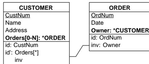
**Figure 7-10:** Object classes, object-attributes and inverse constraint. Note that Orders is a multi-valued identifier of CUSTOMER. Indeed, each order has one owner only, which means that an order identifies its customer.
