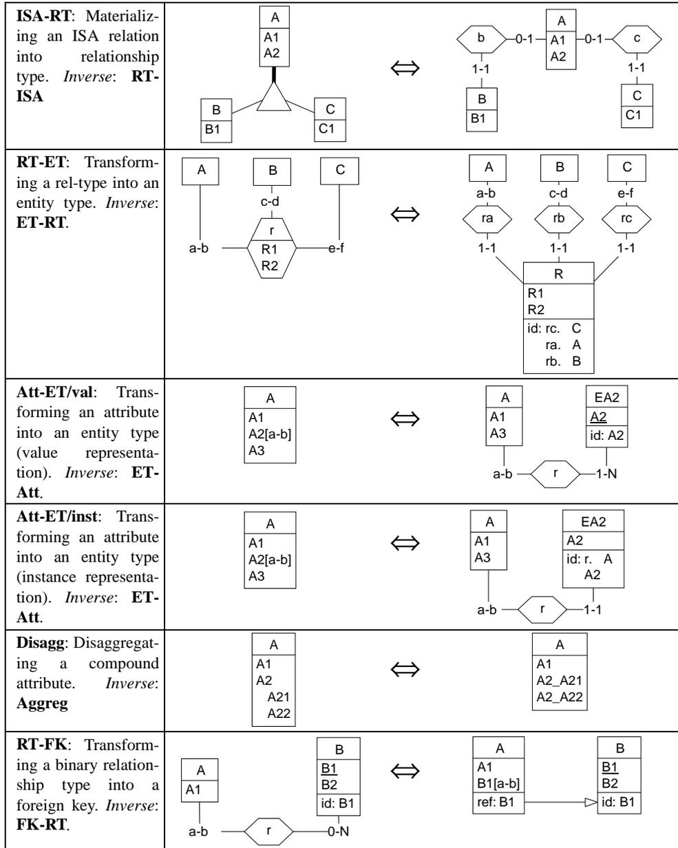
**Figure 2-5:** Six major generic transformations with their inverse. Cardinalities a, b, c and d must be replaced with actual values.
