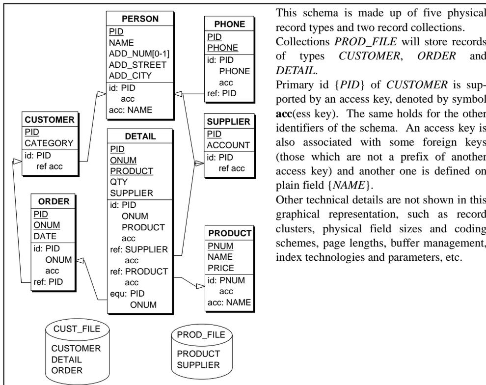
**Figure 2-3:** Abstract physical structures. This schema derives from the logical schema of Figure 2-2.
