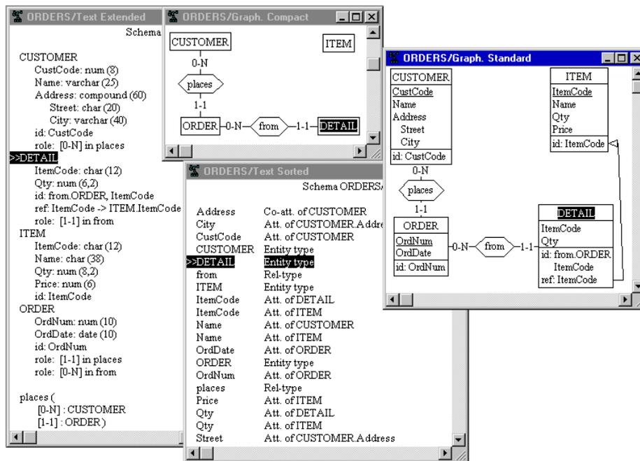
**Figure 8-1:** Four representations of the same schema: text extended (left), text sorted (bottom), graphical compact (top) and graphical standard (right).
