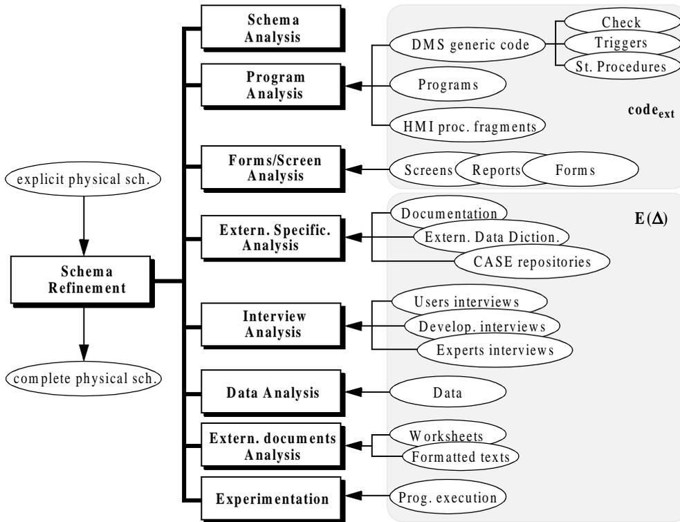
Figure 5-3: Detail of the Schema Refinement process.
