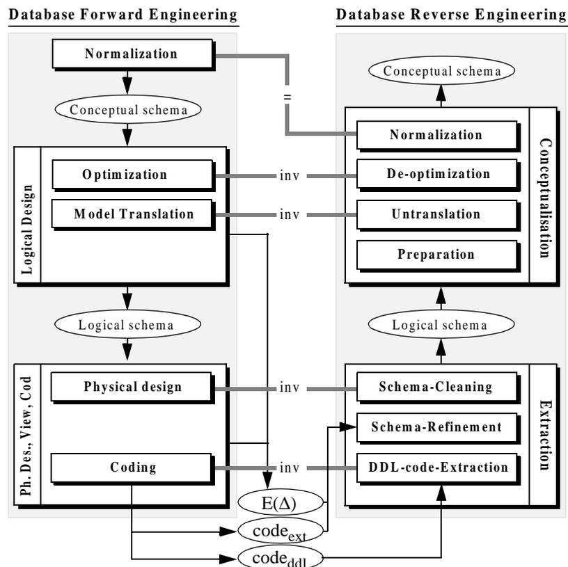
**Figure 4-1:** The main DBRE processes as the inverse of forward processes. Symbol **inv** on the forward/reverse correspondences means that each process is the inverse of the other, while symbol **=** indicates they are the same.
