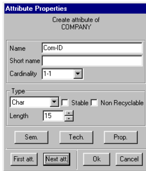
Figure 1.10 - The first attribute of COMPANY is defined. The next attributes will be defined by pressing the Next att. button, or more simply by pressing the Enter key.
