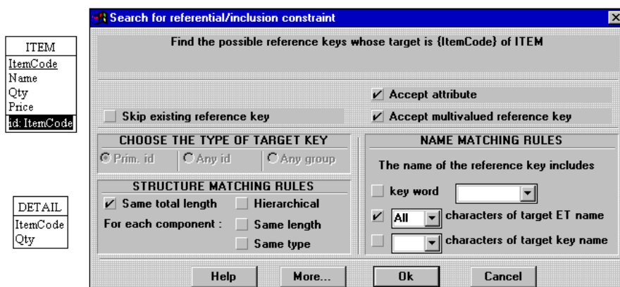
Figure 8-2: Control panel of the search engine of the Reference key assistant of DB-MAIN. Considering a selected identifier (left), it has been asked to find all the attributes, possibly multivalued, that have the same total length, and whose name includes all the characters of the target entity type, i.e. "ITEM". The master panel will then show all the candidate foreign keys, including ItemCode , and propose to define one or several of them.
